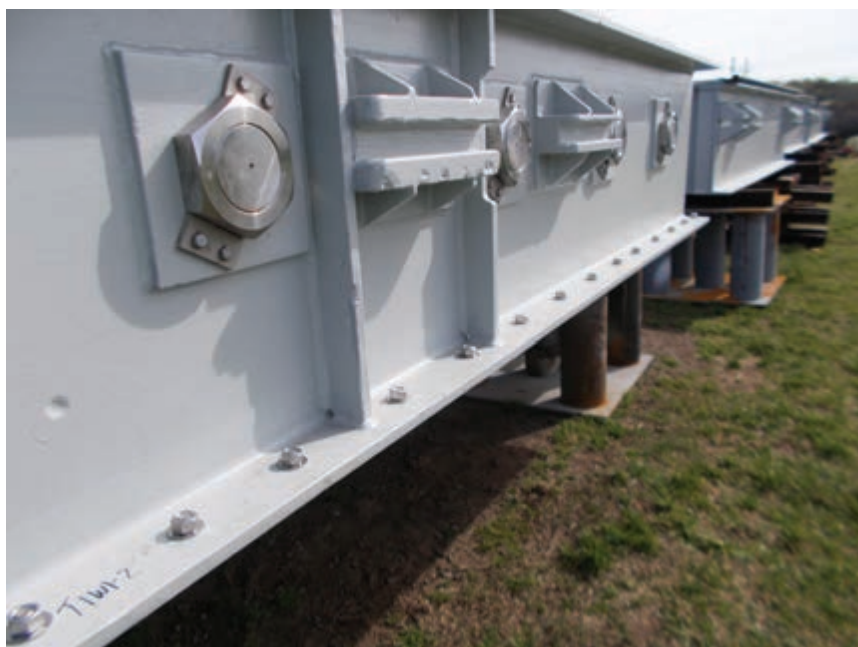
FIG. 4: Intake and tailrace pieces received two stripe coats and three full coats of a polyamide epoxy coating.
